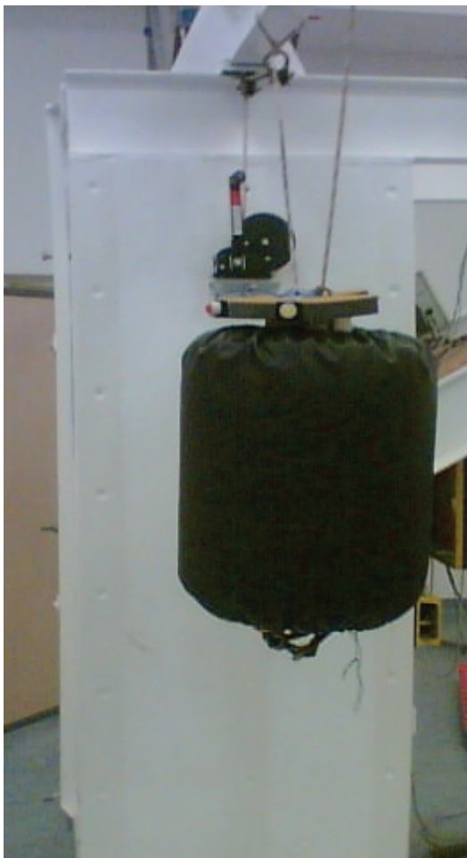
Fig. 1. BTS-3 dynamometric punching bag with an embedded strain gauge
