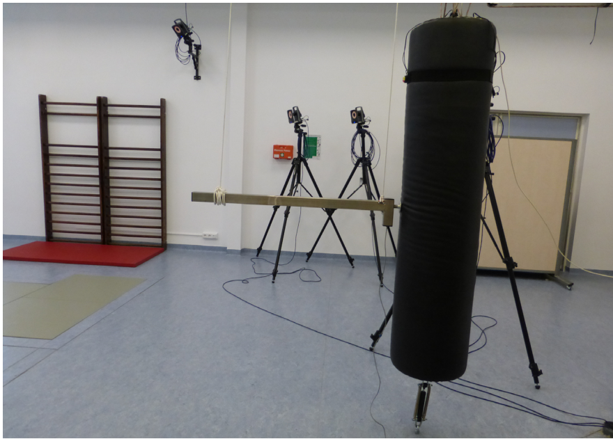
Fig. 4. The view of the dynamometric punching bag having an embedded accelerometer when delivering test strikes
