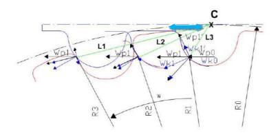
Fig.5. Movement of the teeth in the coupling.
