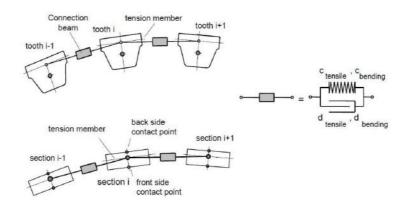
Fig. 3. Rigid body representation of synchronous and non-toothed belt [6]
