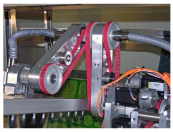
Fig. 2. Timing belts in robotics [15].
