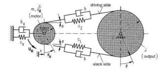
Fig. 4. Schematic representation of the power transmission with timing belt [Dressing H., Holzweissig F., 2010]
