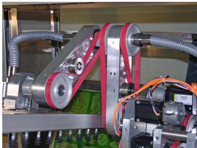
Fig. 2. Timing belts in robotics [15].
