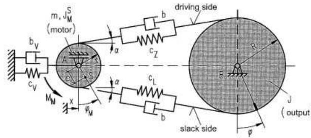
Fig. 4. Schematic representation of the power transmission with timing belt [Dressing H., Holzweissig F., 2010]
