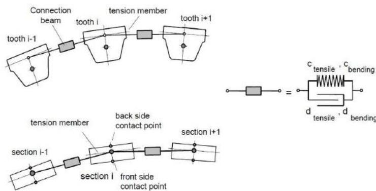
Fig. 3. Rigid body representation of synchronous and non-toothed belt [6]
