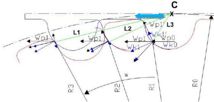
Fig.5. Movement of the teeth in the coupling.
