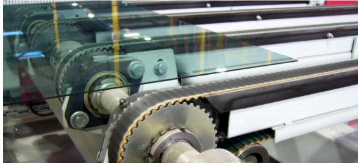
Fig.11. Belts cut from the same sleeve in parallel conveyor
