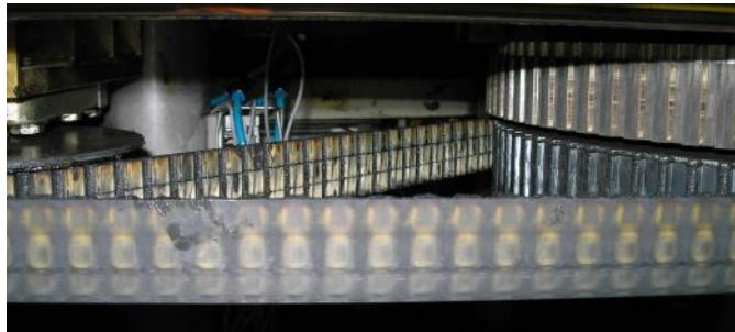
Fig. 10. Belt with pitch accuracy correction at the periphery in control system
