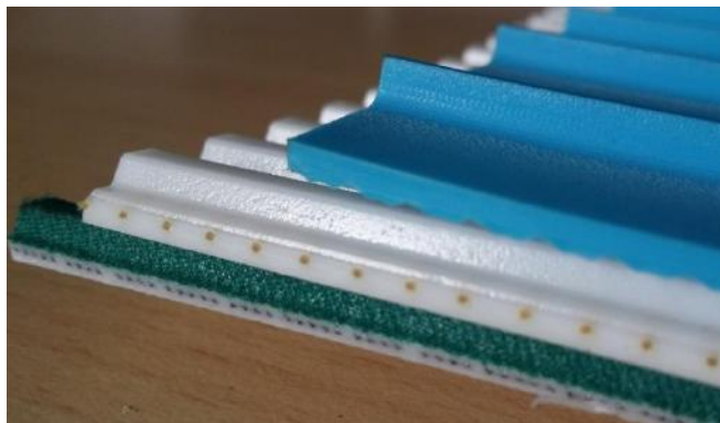
Fig. 3. Examples of timing belts with different constructions of support layer.
