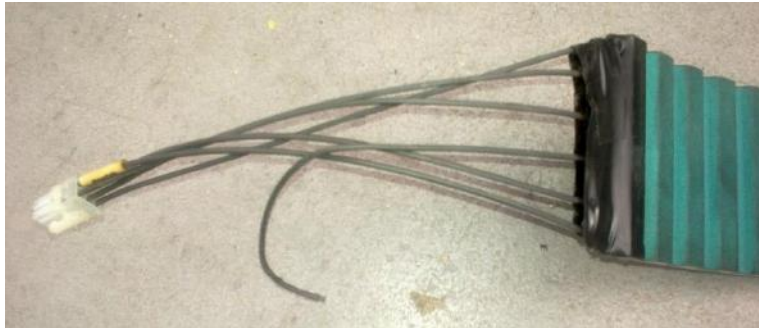
Fig. 4. Timing belt with signal cable.
