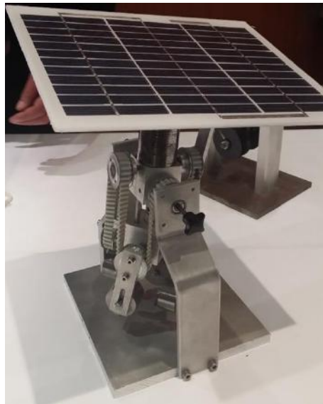
Fig.1. Timing belt for solar panel control.
