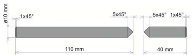
Figure. 6 Selected geometry of the weld surface of the specimen
