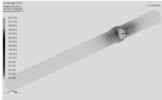
Figure. 3 The simulation of the TIG-welding of the specimen created in the SysWeld program, the temperature gradient in the time t = 0,5 s
