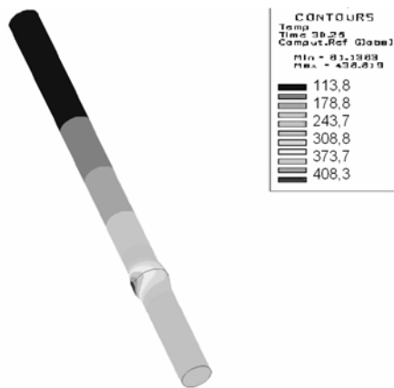
Figure. 8 The temperature gradient during the welding in the time t=30, 5 s
