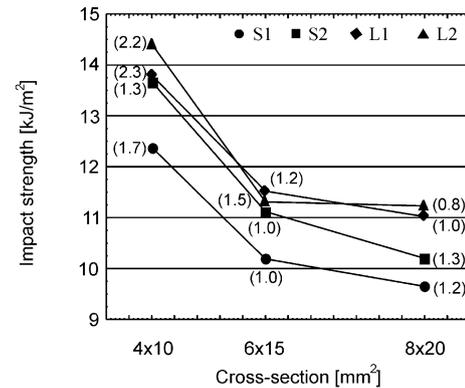
**Fig. 6** Effect of specimen cross-section size on impact strength of WPC with different sizes of wood particles (standard deviations in parentheses)
