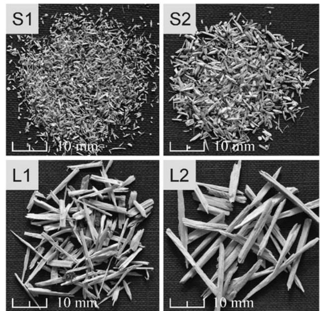
**Fig. 1** Screened wood particles of S1, S2, L1 and L2 sizes
